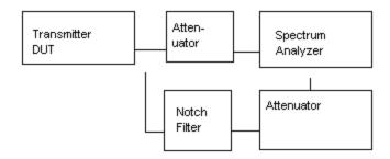
Method of Measuring Conducted Spurious Emissions
