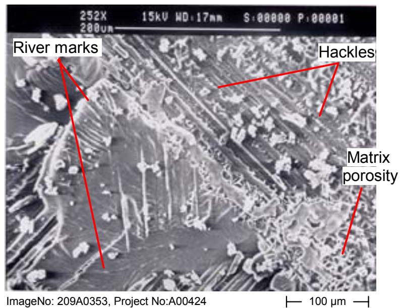
Figure 57. Example SEM photograph from the top forward corner of specimen LF3a-5b. Hackles indicated point up and forward, and river marks also point generally up and forward. Orientation as in figure 56.
