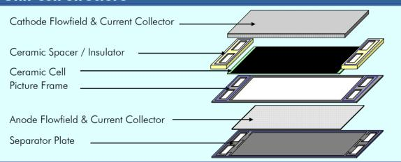
1 Stacks based on planar, rectangular cells shown here; the study assessed three other stack technologies
