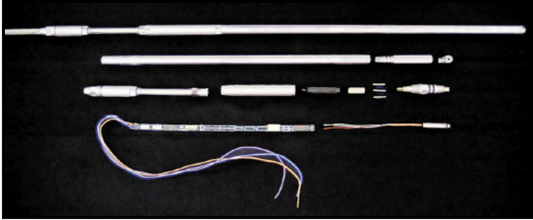
Figure 3: Downhole Pressure/Temperature Gauges for Instrumented Wellbores
