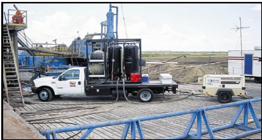
Figure 2: Skid-Mounted Cement Pulsation Unit Operating on Location
