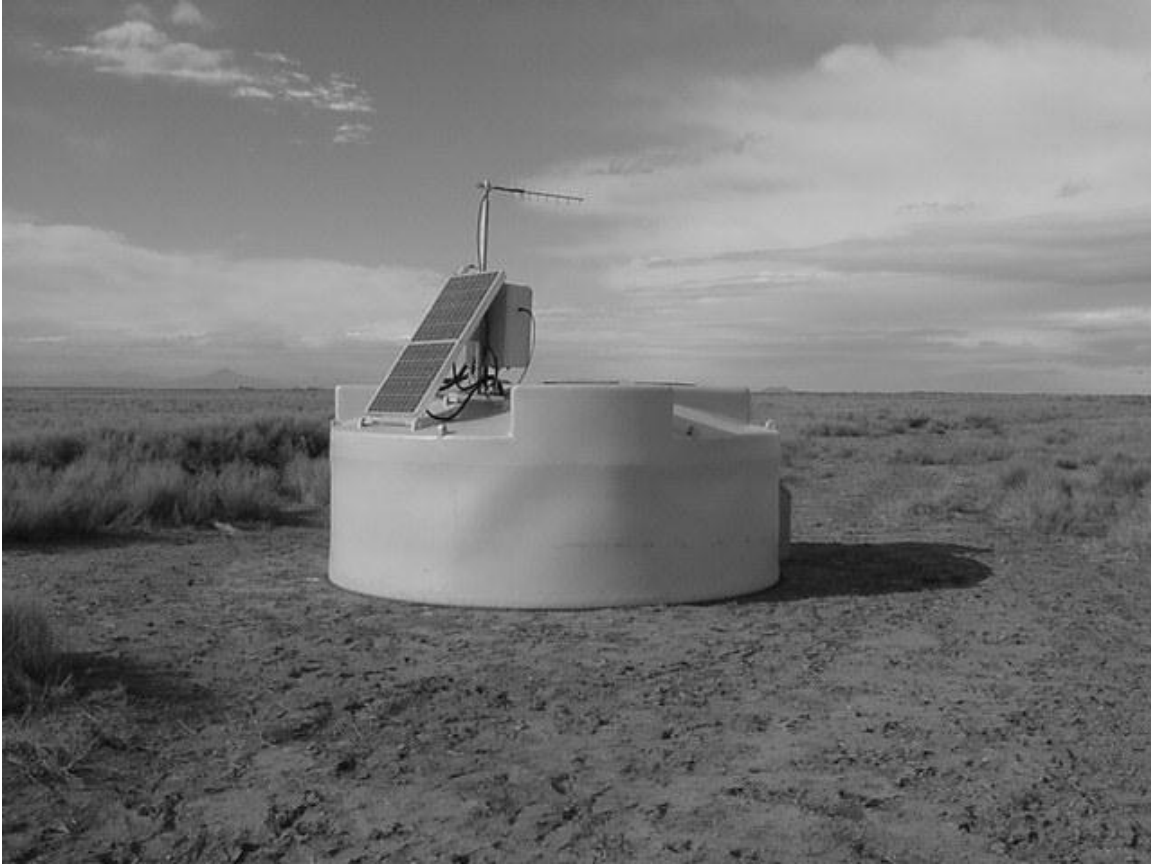
Figure 2.2: A surface detector deployed in the EA. Mounted on top of the tank are the solar panel, electronics enclosure, mast, and antenna.
