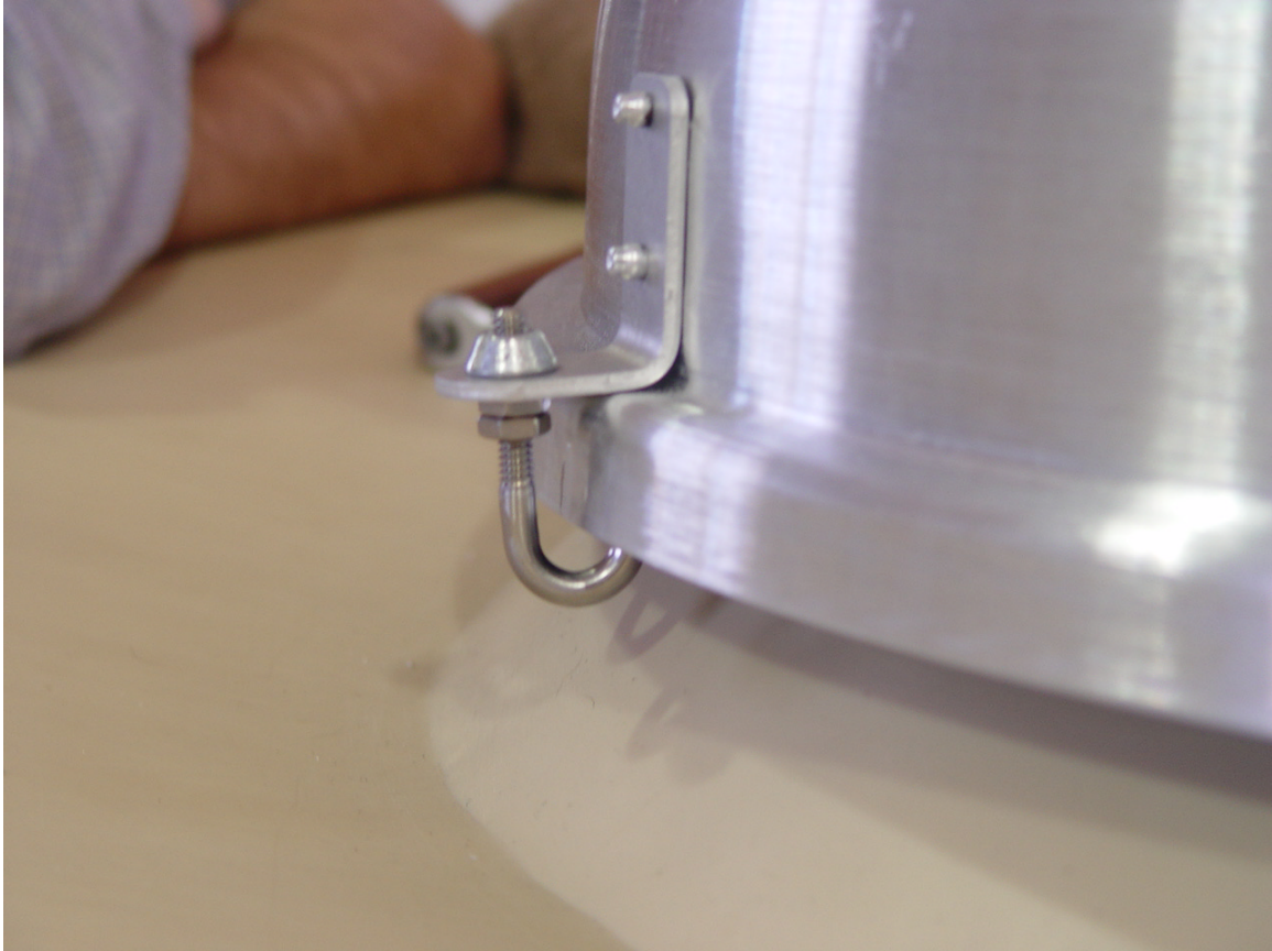
Fig. 2.4. The hold-down system for the weather enclosure consists of a bracket riveted to the dome, a J-bolt which engages the large hatchcover, and two jam-nuts and one security nut, which can be opened only with a special tool.
