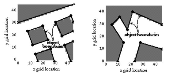
Figure 9: An example set of object boundary curves with the resultant occupancy grid overlaid
