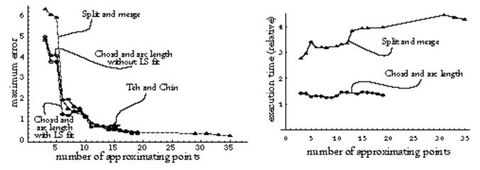
Figure 4: Maximum errors as a function of the number of approximating points for several algorithms using the digital (unsmoothed) curve of Figure 3.
