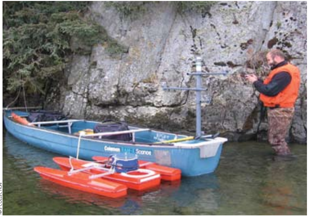
USGS hydrologist installing gauging station at Lake Brooks outflow, Katmai National Park.
