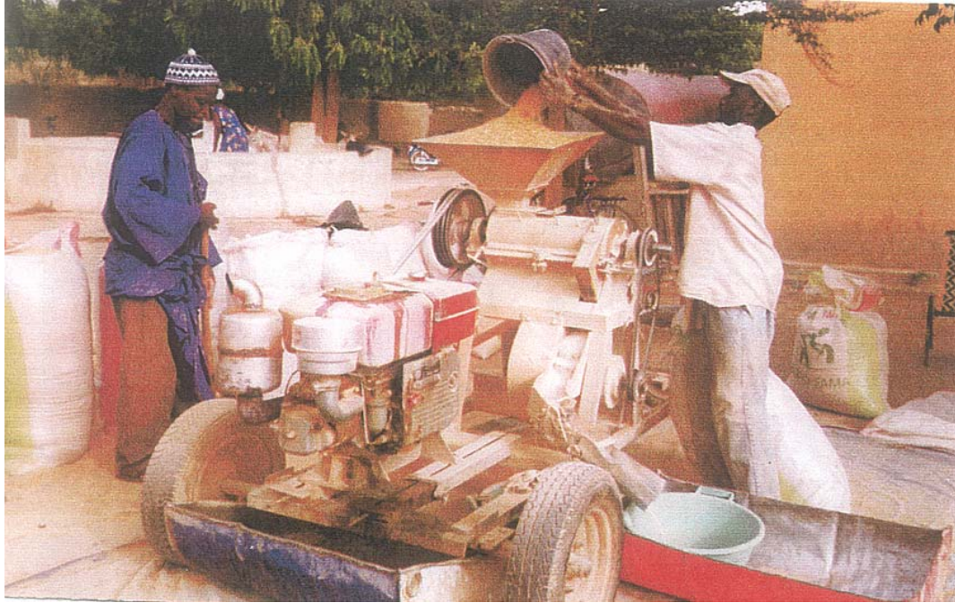
Photo 2 : A traditional husking machine in operation at KM 30
