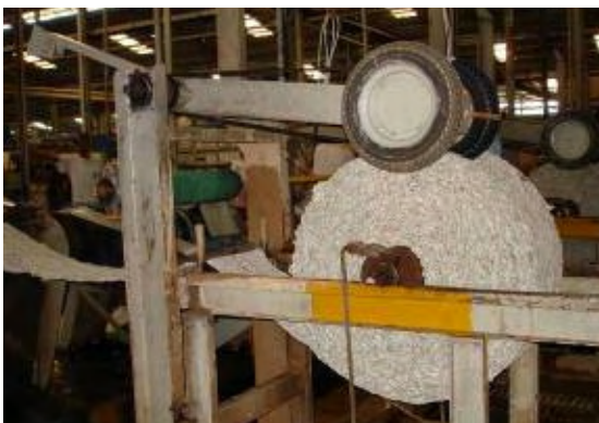
Figure 22 Preparation of wet blankets
