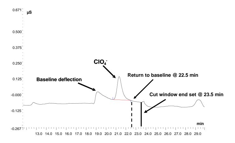
Figure 5. Setting the stop time for the cut window in the first dimension using a 4.0-mL injection volume of a  $10 \mu g/L \text{ ClO}_4$  fortification in RW.
