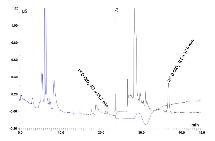
Figure 7. Typical First- and Second-Dimension Chromatograms of a municipal surface water disinfected with chlorine. The native level of perchlorate was  $0.055~\mu g/L$ .
