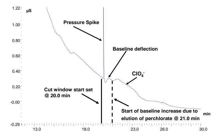
Figure 4. Setting the stop time for the cut window in the first dimension using a 2.0-mL injection volume of a 25  $\mu$ g/L ClO<sub>4</sub> fortification in RW.
