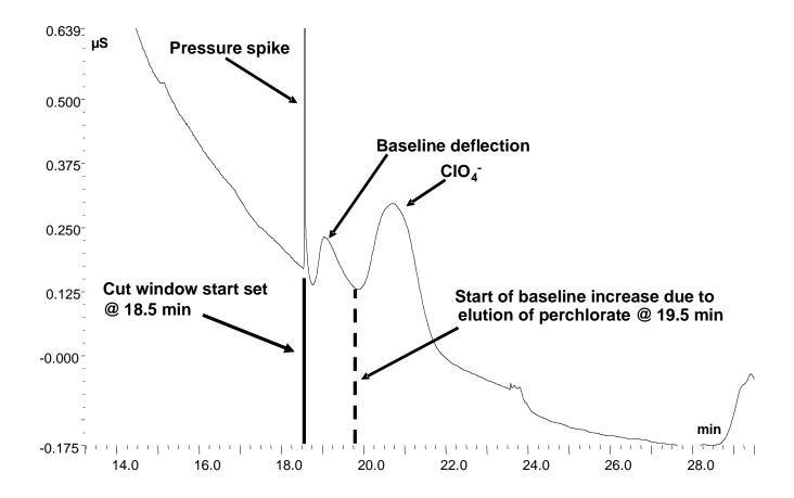
Figure 3 . Setting the start time for the cut window in the first dimension using a 4.0-mL injection volume of a 25  $\mu$ g/L ClO<sub>4</sub> fortification in the 1000 mg/L LSSM.
