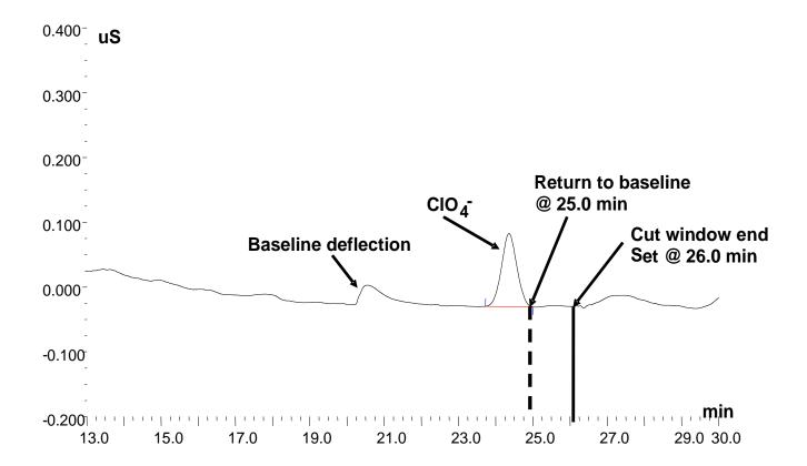
Figure 6. First- and Second-Dimension Chromatograms of 5.0  $\mu\text{g}/L$  perchlorate fortification in Reagent Water.
