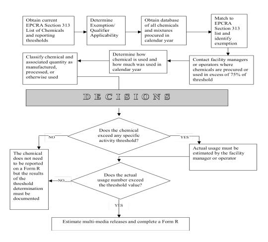
Figure 1. Flowchart process of analysis for EPCRA Section 313 reporting.
