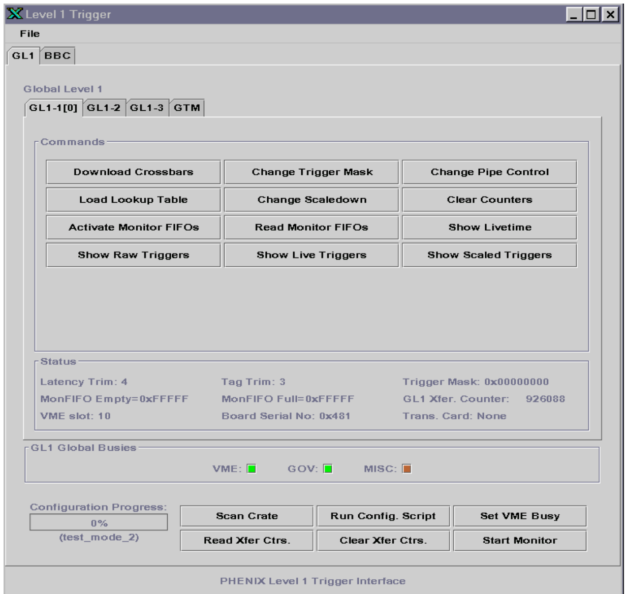
Figure 11: The GL1 gui crate configuration window. Commands are accessed using the buttons under the Options heading or by the menu headings in the upper left. Configuration pages for different elements can be accessed using the buttons directly above the PHENIX logo.
