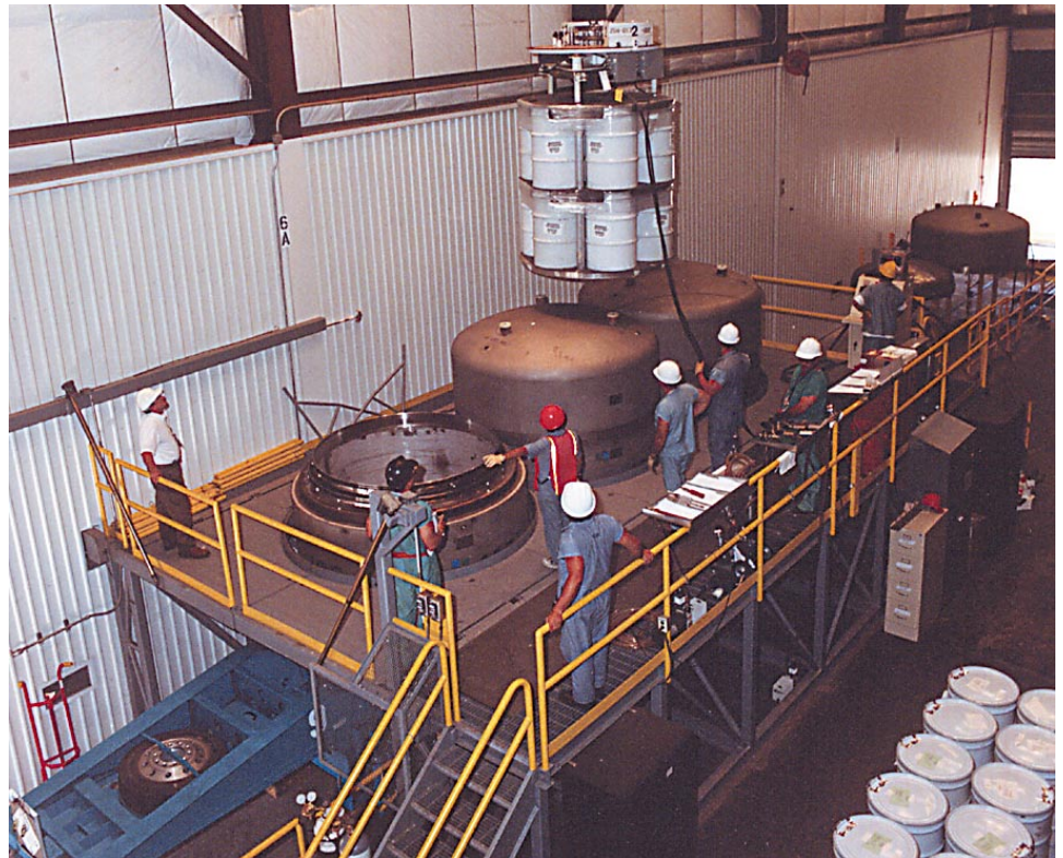
Figure 3: Workers Load 14 of the 55-Gallon Transuranic Waste Drums Into a Transportation Cask
