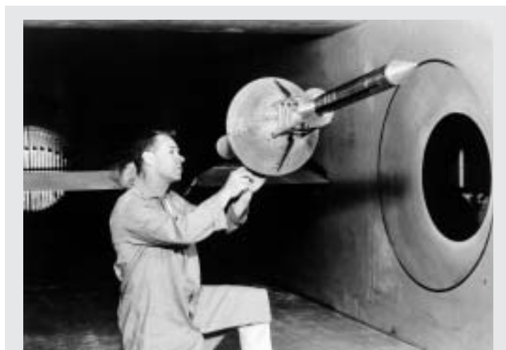
Apollo launch escape system being tested in the Ames unitary wind tunnel, 1963.
