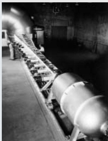
Atmospheric entry simulator, 1959, used to determine if a specific shape can survive atmospheric re-entry.
