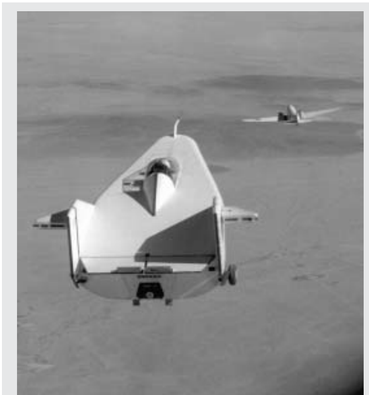
M2-F1 lifting body, shown in a tow test at Dryden in 1964, set design parameters for the shuttle orbiter.
