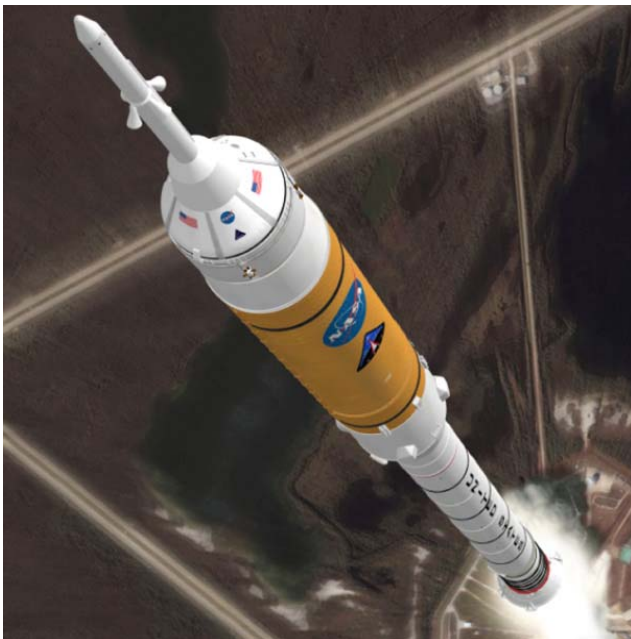
Figure 2 – Ares I Launch Vehicle. The Ares I will incorporate technologies from the Space Shuttle solid rocket boosters and external tank in its first and second stages.
