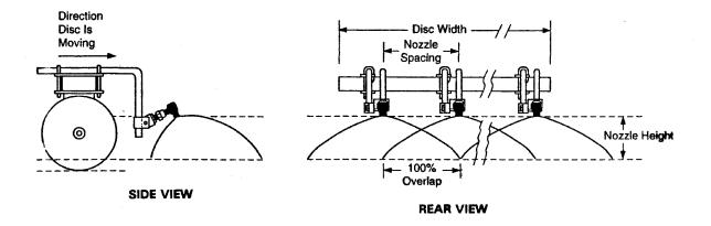
Figure 9.2.1-2. Side view and rear view of a typical spray nozzle system used for application of fluid fertilizers.
