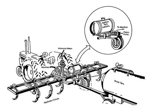
Figure 9.2.1-1. Typical trailer for application of anhydrous ammonia and fluid fertilizers.
