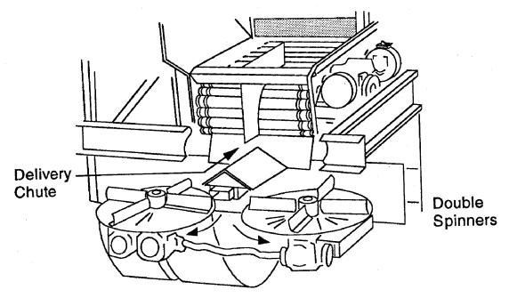
Figure 9.2.1-3. Example of centrifugal spreader.
