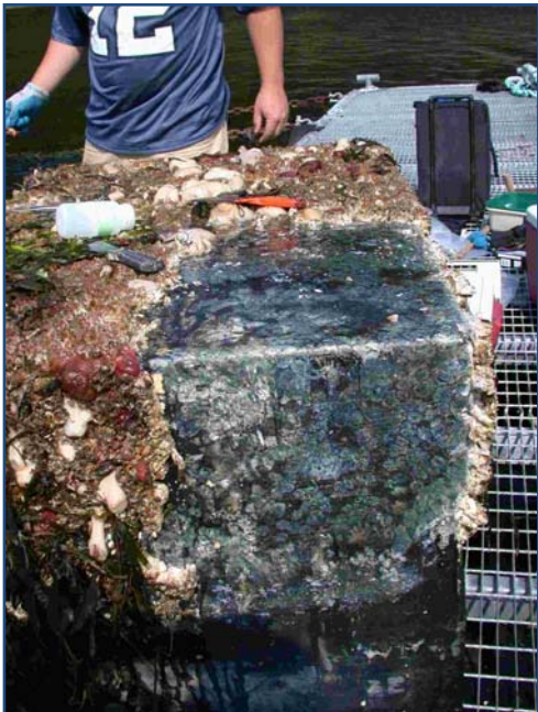
Figure 6. Sampling by scraping biocolonization from different surfaces of a net pen float.
