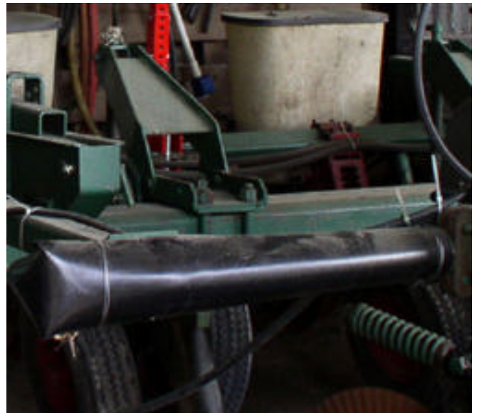
This picture shows how Jeff uses black plastic pipe and pvc pipe to keep residue from hanging on the tool bar and coulter in no-till planting.
