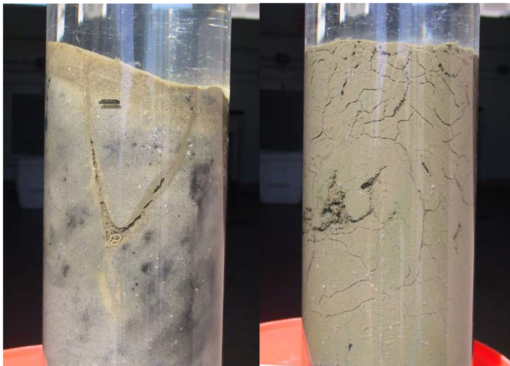
Figure 6. Effects of burrowing organisms on sediment cores. Core on left contains a large brittle star with its disk approximately 5 cm below the sediment surface and its arms stretched upward through the sediment into the overlying water. Core on right contains numerous small polychaetes which irrigate the sediment during incubations.
