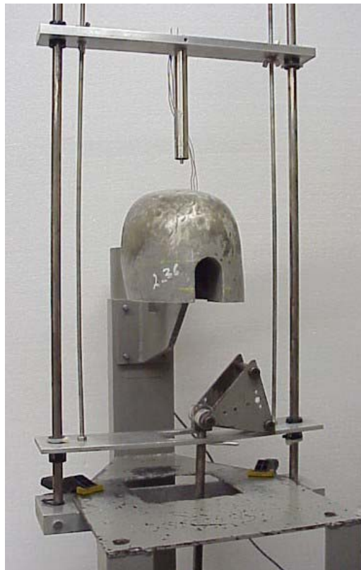
SwRI Helmet Test Equipment Photo 6. Retention System Tester with Supported DOT Headform, Simulated Jaw, and Displacement Measuring System
