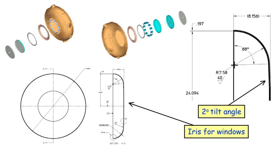
~ 6 mm Cu plates, spinning + e-beam welding
