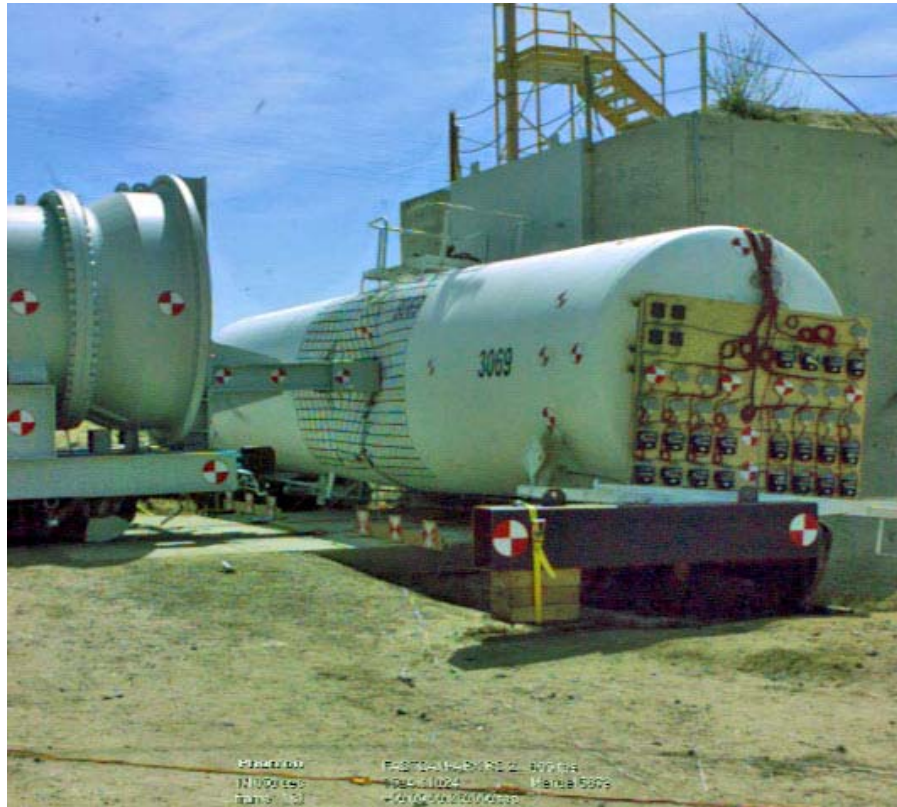
Large Impactor Face Does Not Rupture Tank
