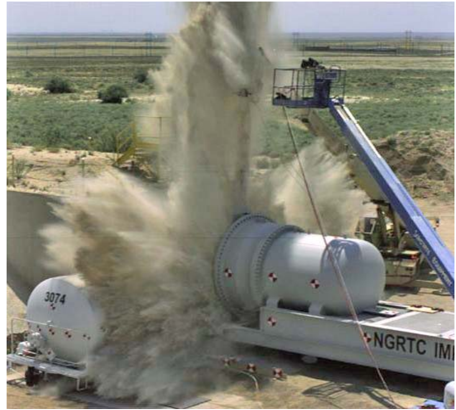
Small Impactor Face Ruptures Tank
