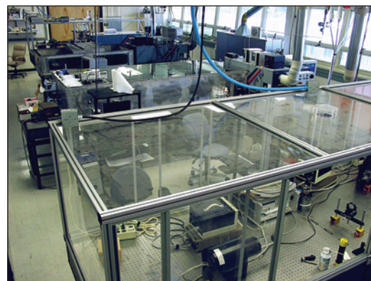
Figure 2. Laboratory for excimer laser energy and power meter calibrations, with measurement systems for 248 nm, 193 nm, and 157 nm. The excimer lasers are along the top right and the enclosures for nitrogen gas purging are in the foreground.
