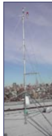
Instruments that measure winds and temperatures in the city and above building tops.
