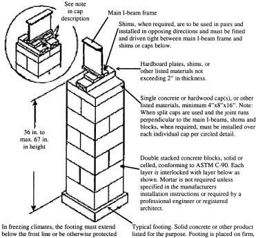
In freezing climates, the footing must extend below the frost line or be otherwise protected from the effects of frost heave as permitted here-in.
