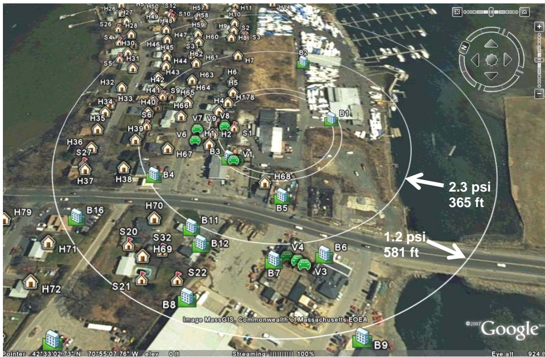
Figure A-1. Aerial view showing damage data points and estimated explosion overpressures. CAI/Arnel facility is in the double circle, center. (graphic: Google Earth Pro)
