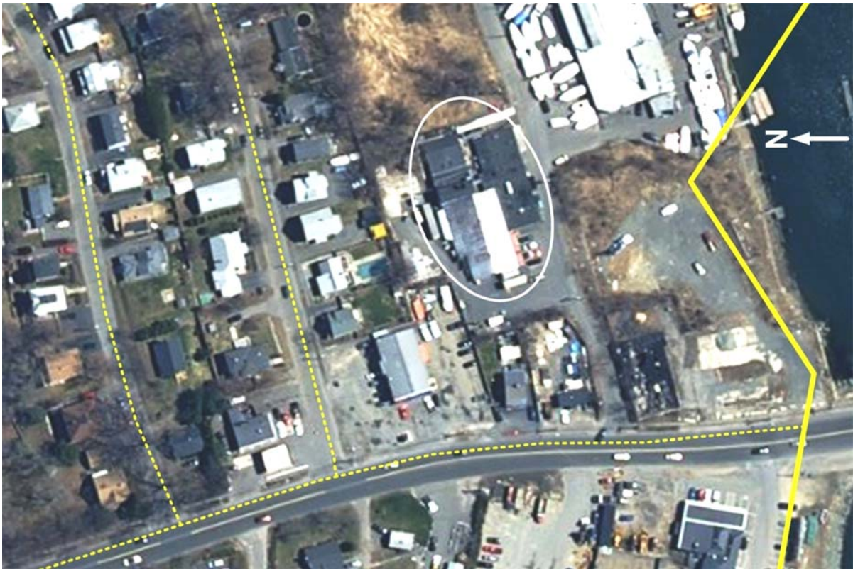
Figure 18. Buried natural gas lines near the CAI/Arnel property (circled). Solid line – Maritimes and Northeast pipeline. Dashed line – KeySpan utility pipeline.
