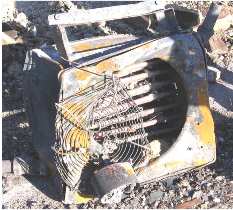
Figure 4. Steam coil air heater recovered from the debris. Fan motor is at the lower center of the photo.
