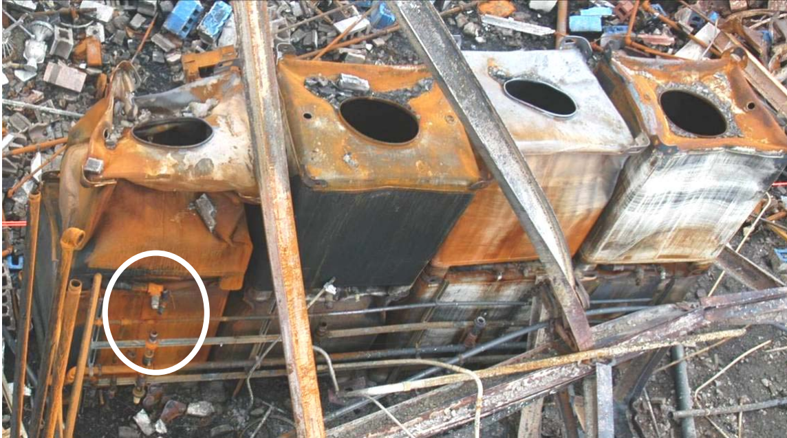
Figure 7. CAI totes stored flammable liquids in area E. Circled area shows one of the flexible hose connection points to the manifold pipe.
