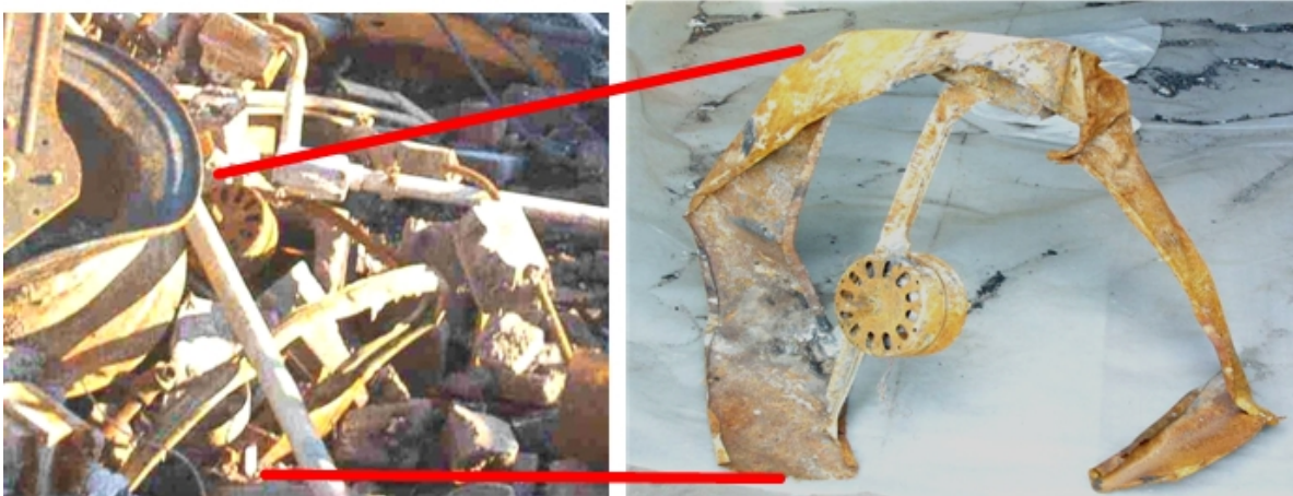
Figure 22. Box fan, a possible ignition source recovered from the debris near area E.
