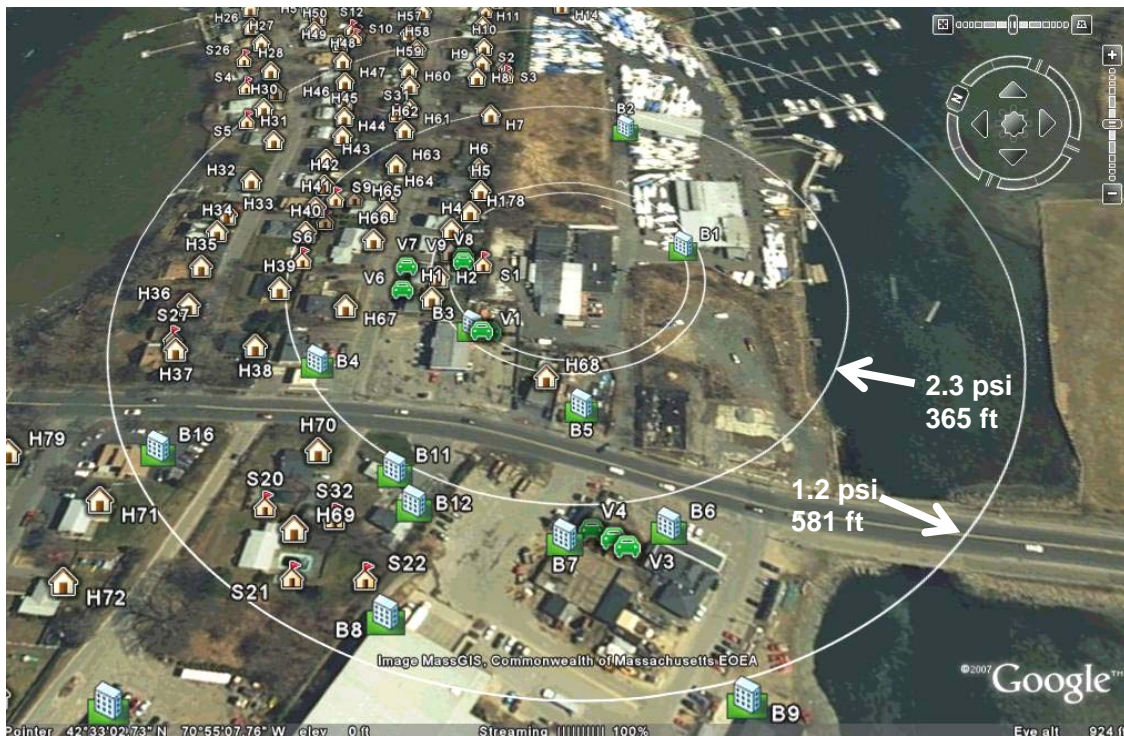
Figure 20. Aerial view showing some damage data points and estimated explosion overpressures out to about 600 feet from the facility (double circle, center). Google Earth Pro
