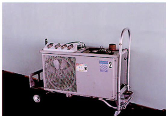
Figure II-07 Air Compressor, Bauer Mariner
