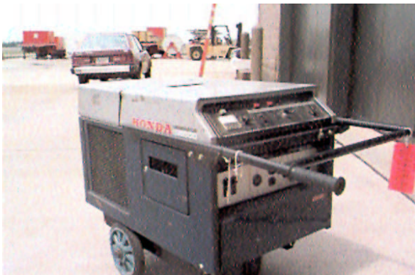
Figure II-13 Generator, 5.5 kW, Honda
