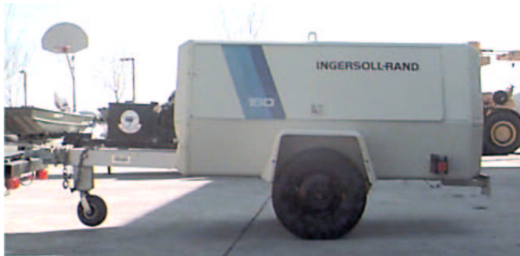
Figure II-08 Air Compressor, Ingersoll Rand
