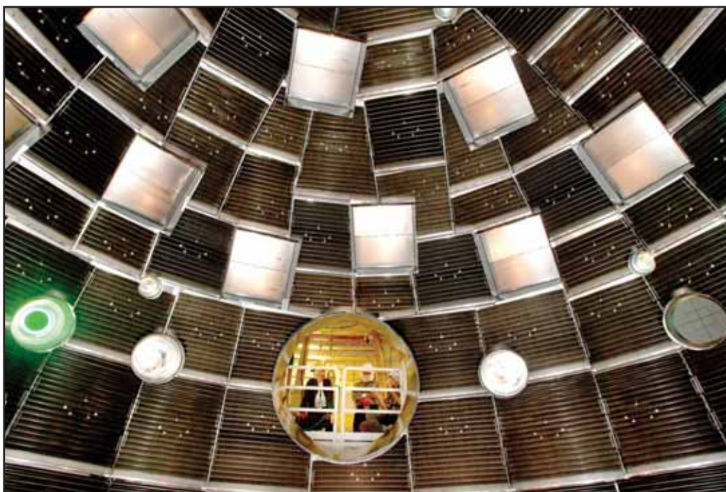
Researchers peer into the NIF target chamber, with its newly installed protective wall. The laser surpasses another milestone — on its way to beginning ignition experiments in 2010.
