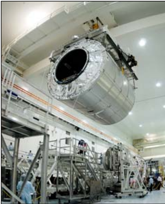
Multi-Purpose Logistics Module Raffaello in the Space Station Processing Facility. Raffaello is the second MPLM built by the Italian Space Agency, serving as a reusable logistics carrier and primary delivery system to resupply and return station cargo requiring a pressurized environment.
