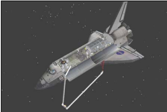
Orbiter Boom Sensor System (OBSS) inspects reinforced carbon-carbon of wing leading edge
