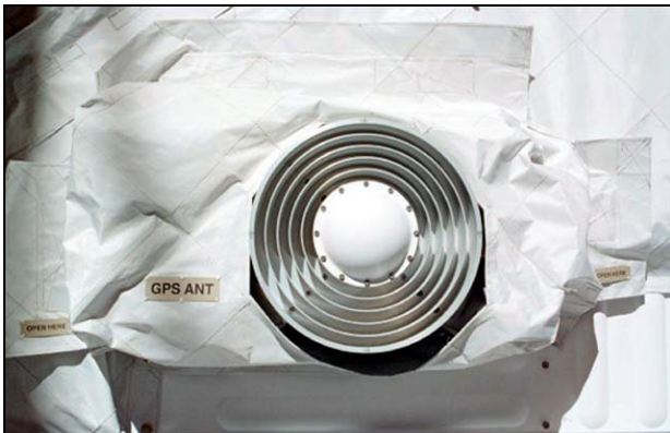
A Global Positioning System (GPS) antenna (above) and its location on the International Space Station truss (below)
