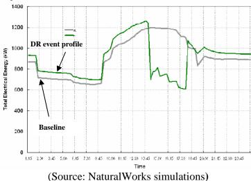
Figure 4. Preliminary Results on Total Demand Profile of the NYT Occupied Tower Floors
