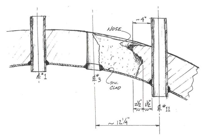
The above figure shows the Davis Besse reactor vessel head degradation between nozzle #3 and nozzle #11. This sketch was provided to the NRC by the Licensee.
