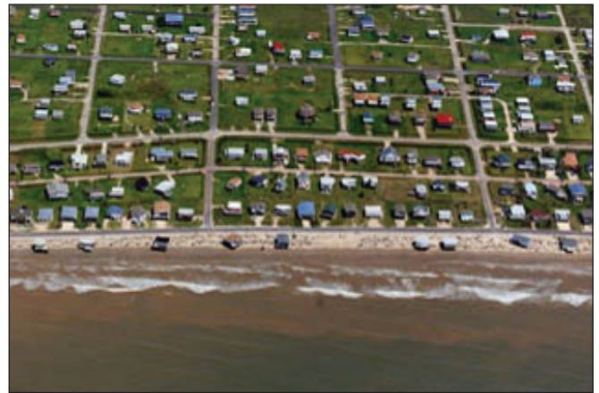
Figure 2. Long-term erosion has caused the shoreline to retreat and has left homes standing on the beach (Surfside Beach, TX). July 2007 Texas General Land Office photo.
