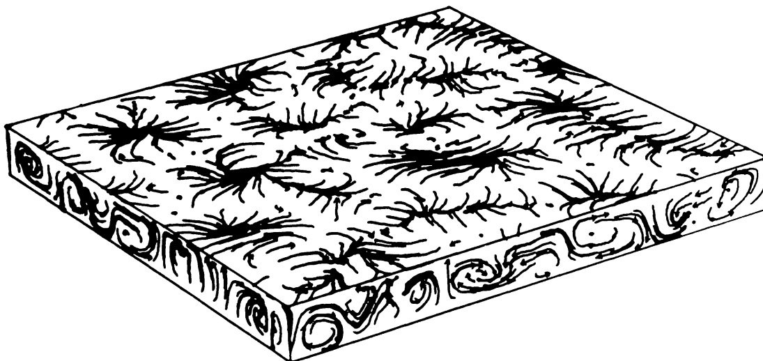
Fig. 2. Particle trajectories in three orthogonal planes for the final time step at 90^\circ latitude. The three-dimensional pattern consists of cells with diameters of 30 000 to 50 000 km. The flow on the top surface is from the updrafts (open regions from which the lines diverge) to the downdrafts (dark regions where the lines converge).
