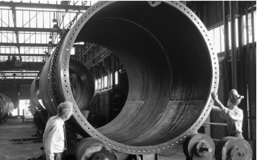
Figure 9.5 Manufacturing towers for Enercon turbines, Western Australia
