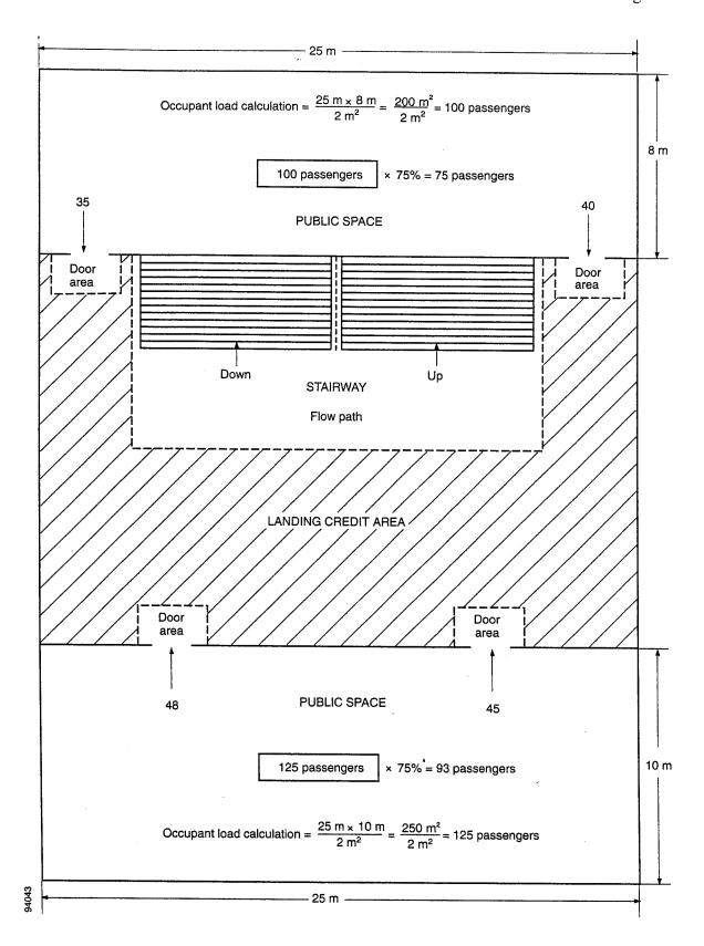
Figure 3 - Occupant loading calculation example
