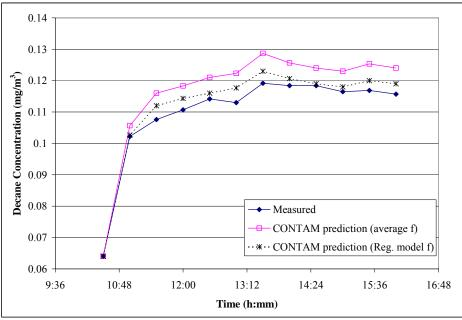
Figure 1. Comparison of measured and predicted decane concentrations
