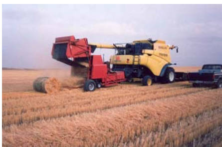
Figure 3. Feedstock collected by single-pass multi-component harvester, 2003.
