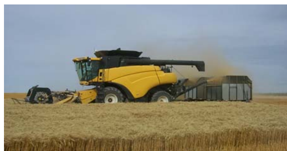
Figure 2. INL two wagon harvesting system, 2004.
