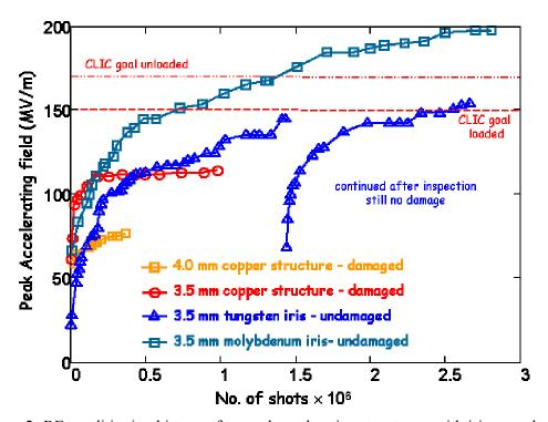
**Figure 2:** RF conditioning history of several accelerating structures, with irises made of different materials and with different apertures, tested with beam in CTF2.
