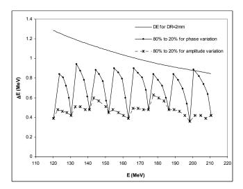
**Figure 6:** Energy spread due to phase modulation and amplitude modulation. The energy spread is defined considering the distribution in energy of the accelerated beam and by keeping the distance in energy between 80% to 20% of the beam in such distribution.
