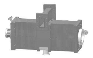
**Figure 5:** The first module of LIBO-30; the wave-guide brazed on top of the central bridge-coupler feeds the two tanks.
