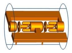
**Figure 1:** Channel of an RFQ-DTL, length βλ.
