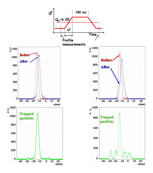
**Figure 16:** Results of the dependence of the beamlets parameters on the resonance crossing speed. The sketch of the measurement principle is shown in the upper part. The horizontal profiles for a fast crossing (5 ms) are shown in the left part, corresponding to the three moments, while the profiles on the right correspond to a slow crossing (90 ms). The fact that the profiles are not centred at zero is due to an instrumental offset of the wire position.
