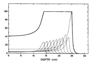
**Figure 2:** SOBP composed of doses delivered at different energies (dotted Lines).
