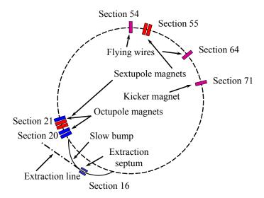
**Figure 11:** Schematic layout of the PS machine with the elements used for the experimental study of the novel multi-turn extraction.
