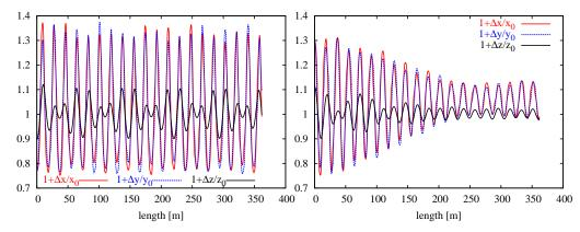
**Figure 3:** Core oscillations for a 6D waterbag/Gaussian (left/right) beam due to the excitation of the fast mode with 30% initial mismatch. (IMPACT [19] simulation with  $10^6$  particles.)
