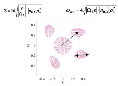
**Figure 6:** Example of islands and their characteristic parameters
