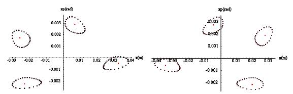
**Figure 4 :** Shape of the stable islands at two straight sections of the PS machine, namely the extraction section (left) and the section where the wire scanner used for profile measurements (see next Sections) is located (right).
