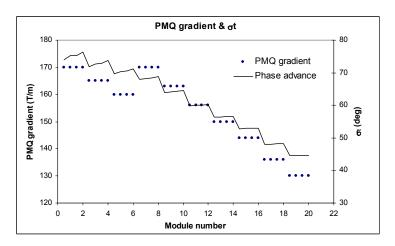
**Figure 8:** PMQ gradient and transverse phase advance per focusing period.
