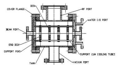
Figure 1: Schematic of a four-cell PWT linac structure.
