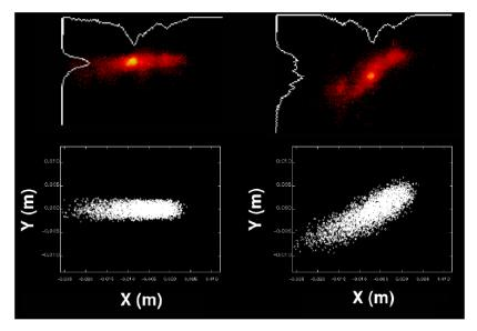
**Figure 8:** Measured (top) and simulated (bottom) transverse beam distributions with the RF deflector off (left) and on (right), for  $R_{56} = 0.1$  m. Horizontal dispersion at the location of the screen is responsible for the correlation visible in the images to the right (from C. Biscari, INFN/LNF).
