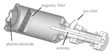
Figure 5: Prototype volume production, RF excited, negative hydrogen ion source
