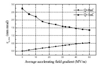
**Figure 4:** Emittance at the exit of the four-cell PWT linac, as a function of accelerating gradient.
