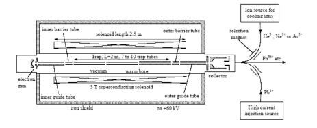
Figure 7: Conceptual confined flow EBIS with external injection
