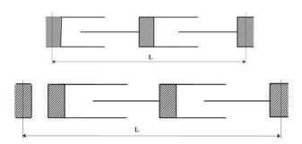
**Figure 3:** Examples RFQ-DTL layouts with one and two spacer electrodes.
