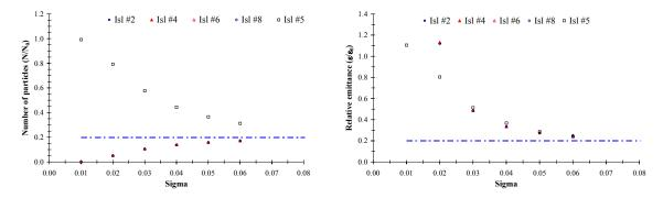
**Figure 5:** Results of numerical simulations to evaluate the intensity trapped in each island vs. the sigma of the initial bi-Gaussian distribution (left) and the emittance of each beamlet vs. the sigma of the initial bi-Gaussian distribution (right). The dot-dashed line represents the goal of perfect splitting, i.e. equal intensity and emittance among the five resulting beamlets.
