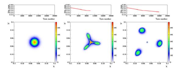
**Figure 8:** Evolution of the beam distribution during resonance crossing: the initial state is represented by a Gaussian beam (left), at resonance-crossing some particles are trapped inside the moving islands (centre), at the end of the process, the particles trapped in the islands are moved towards higher amplitudes (right).
