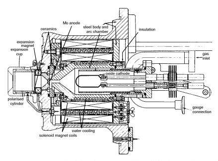
**Figure 2:** CERN standard duoplasmatron (with polarised expansion cup)
