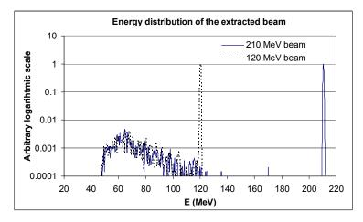
**Figure 10:** Energy distribution of the extracted beam in logarithmic scale.
