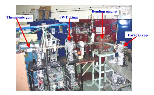
Figure 5: Photograph of the layout of the beam-line for the acceleration experiments
