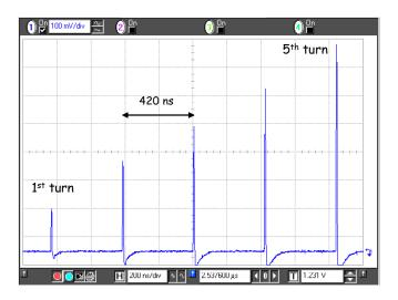
**Figure 3:** Oscilloscope trace from an intensity monitor in the CTF3 preliminary phase combiner ring, showing the increase in circulating beam current over five turns from 0.3 A to 1.5 A.
