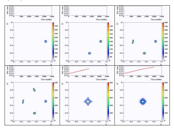
**Figure 10:** Multi-turn injection by means of trapping in stable islands of transverse phase space. Four turns are injected and the beamlets merged by crossing the fourth-order resonance. As a result a hollow beam in the transverse phase space is generated.
