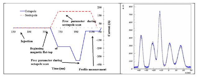
**Figure 14:** Current as a function of time for the sextupoles and octupoles as used in the special test to increase the fraction of particles trapped in the beamlets (left). The resulting horizontal beam profile after splitting is also shown (right). The fact that the profile is not centred at zero is due to an instrumental offset of the wire position.
