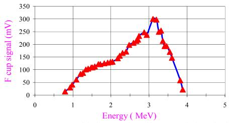
**Figure 6:** Energy spectrum of the beam accelerated in PWT3. The incoming beam is unbunched.
