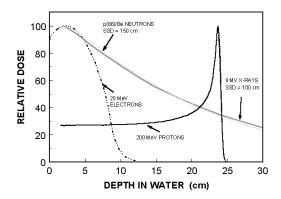
Figure 1: Comparison between photons and protons in water.
