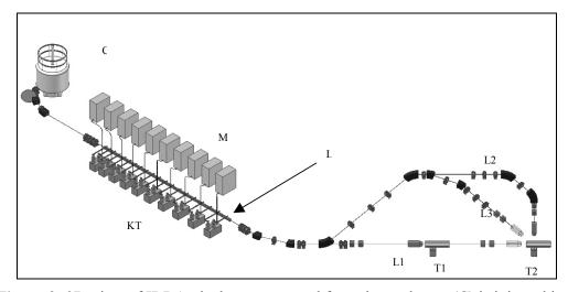
**Figure 3:** 3D-view of IDRA; the beam extracted from the cyclotron (C) is injected into LIBO-30 (L) and, post-accelerated, three extraction lines (L1, L2, L3) distribute it to two treatment rooms (T1, T2). On top of the linac, but in a different gallery, 10 solid-state modulators designed by TERA (M) feed 10 double klystron high voltage oil tanks (KT); the RF power generated by the 20 klystrons is then delivered to the 20 modules of LIBO-30 (L) via wave-guides.
