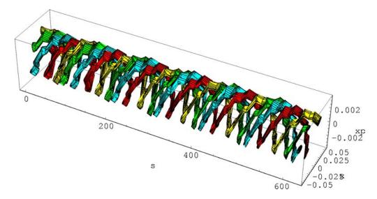
**Figure 3:** 3D view of the beamlets along the circumference of the CERN-Proton Synchrotron (PS) machine. The fifth beamlet, i.e. the beam core, is not shown here.
