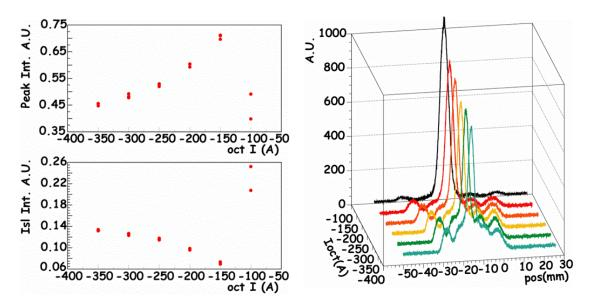
**Figure 17:** Results of the influence of the octupolar strength on the fraction of particles trapped in the beamlets (upper left) with respect to the intensity in the central core (lower left). A series of horizontal beam profiles measured for different values of the octupolar strength are also shown (right part).
