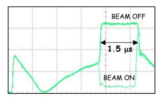
**Figure 7:** Oscilloscope trace showing the RF pulse at the output coupler of a structure. When the beam is on, it extracts more than 90 % of the energy contained in the useful part of the RF pulse (1.5 µs). Virtually no power goes to the load.
