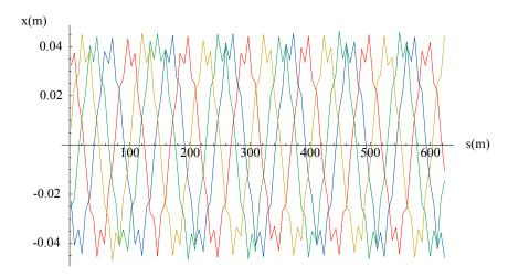
**Figure 18:** Closed-orbit for the four beamlets along the circumference of the PS machine. The closed-orbit of the central core is the origin of phase space.
