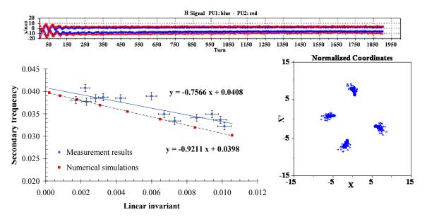
**Figure 12:** Results of the phase space measurements in presence of stable islands generated by means of sextupoles and octupoles. The beam position vs. the number of turn is shown in the upper part, while the reconstructed phase space is shown in the lower right part. The secondary frequency vs. the amplitude inside the island is shown in the lower left part.
