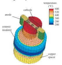
**Figure 2:** Finite element thermal model of the ISIS ion source showing steady state temperatures.
