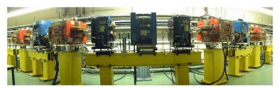
**Figure 6:** The bunch length manipulation chicane.
