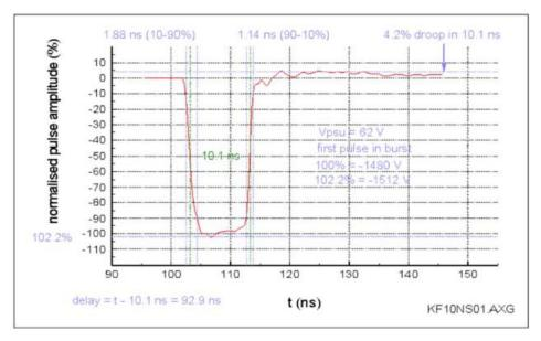
Figure 4: "Fast" chopper pulser waveform into a dummy load.
