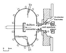
**Figure 3:** Cross section of a steady state magnetron negative ion source
