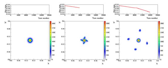
**Figure 2:** Evolution of the beam distribution during resonance crossing: the initial state is represented by a bi-Gaussian beam (left), at resonance-crossing some particles are trapped inside the moving islands (centre), at the end of the process, the particles trapped in the islands are moved towards higher amplitudes (right).
