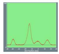
**Figure 13:** Best result achieved with a high-intensity beam, whose intensity as a function of time (left) and horizontal beam profile at the end of the capture process (right) is shown. The fact that the profile is not centred at zero is due to an instrumental offset of the wire position.
