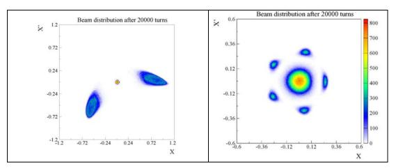
**Figure 9:** Final stage of the splitting process after crossing the half-integer resonance (left) and the fifth-order resonance (right).
