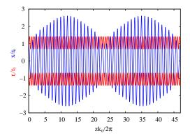
**Figure 1:** Particle trajectories and core envelopes for initial mismatch in a 1D uniform focusing channel with:  $k/k_0=0.8$ ,  $r_c/r_0=0.8$ , x(0)=0.9  $r_0$ .
