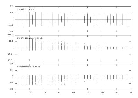
**Figure 7:** The beam evaluated in the middle of the PMQs in the case of full acceleration to 210 MeV. From top to bottom: beam transverse beam profile, phase width and energy spread along the linac.
