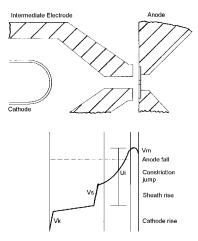
**Figure 1:** Idealised potential distribution in the duoplasmatron discharge
