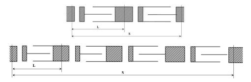
**Figure 4:** Arranging FD and FFDD focusing patterns.
