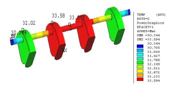
**Figure 2:** Steady-state temperature profile of the disk-array with copper rods.
