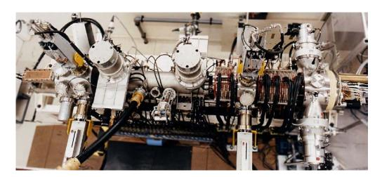
**Figure 3:** The ISIS RFQ test facility. The RFQ pre-injector has now been successfully installed on the ISIS accelerator.
