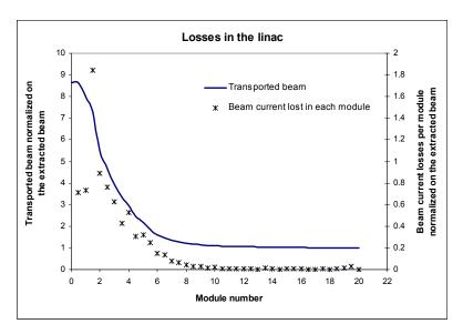
**Figure 9:** The beam losses in LIBO for the case of full acceleration to 210 MeV. For the 66 MeV beam the results are identical.
