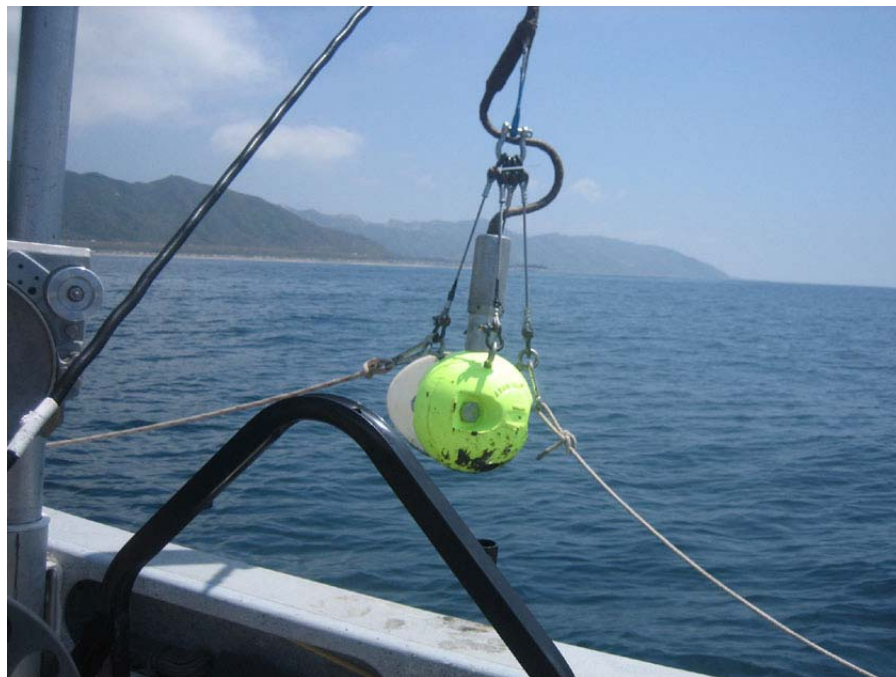
Figure 14. Top: Beachball© camera: digital camera encased in waterproof housing. Bottom: Flying Eyeball©: digital video camera encased in wrecking ball.
