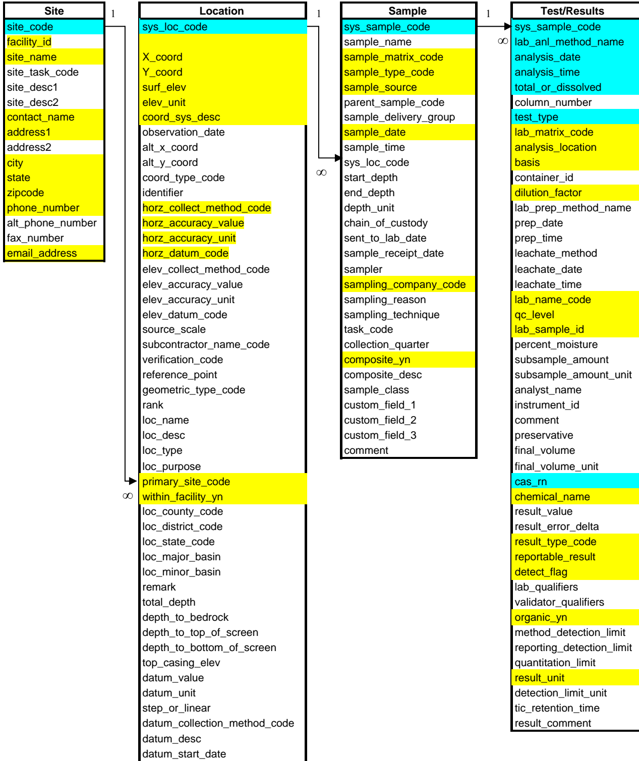
Figure 2-1. Relationships between chemistry file data structures. Shaded fields are required to have data. Blue fields define row uniqueness for the specified file.
