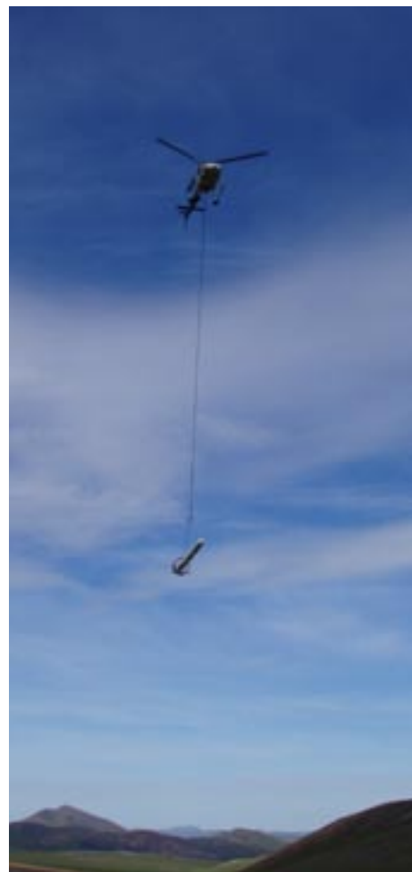
(above) Sensors measure electromagnetic qualities that can help locate concealed mineral deposits.
