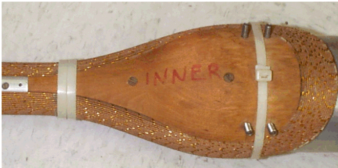
Fig. 2. Dogbone end design for “React & Wind” technology.
