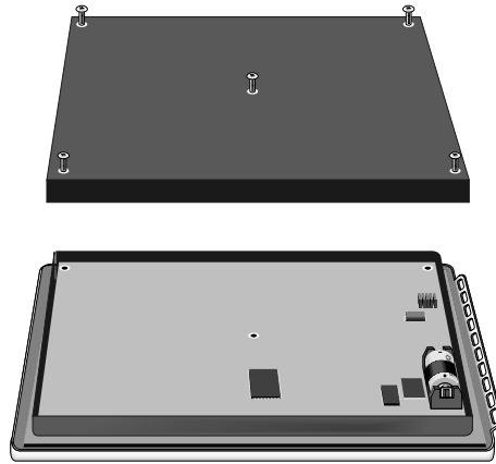
FIGURE 14.10-4. Removal of CR23X back plate and lithium battery location.
