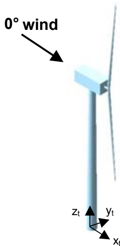
Figure 3. Tower-base coordinate system.
