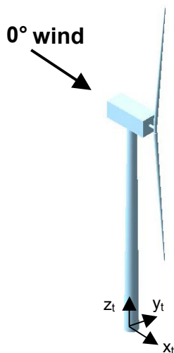
Figure 3. Tower-base coordinate system.
