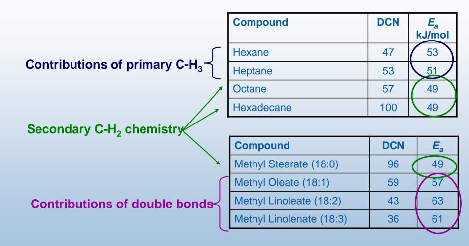
**Biodiesel ignition chemistry dominated by hydrocarbon chain**
