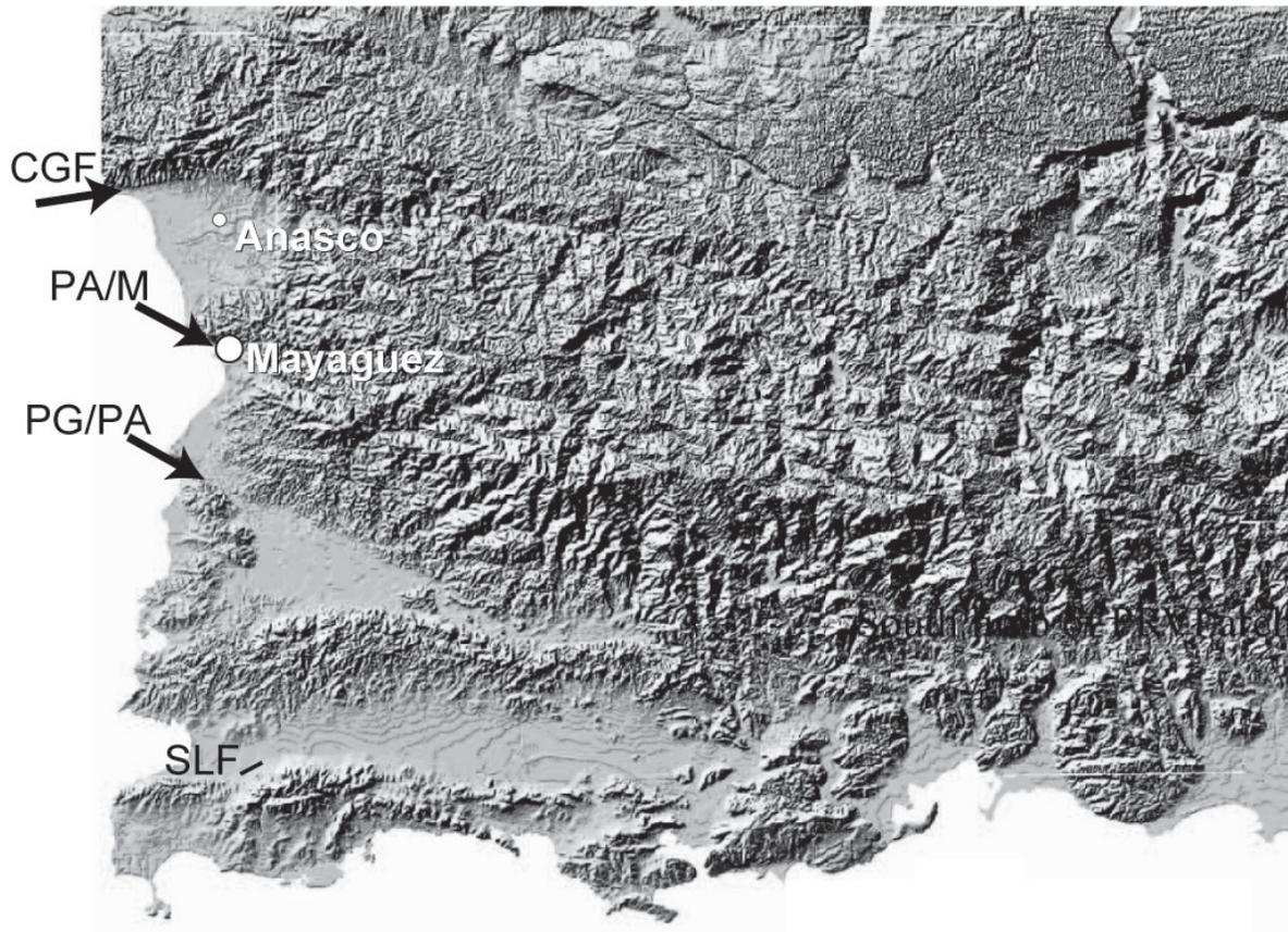
Figure 3. Digital elevation model of western Puerto Rico showing several major faults, including the Cerro Goden fault (CGF), Punta Algarrobo/Mayaguez fault (PA/M) Punta Guanajibo/Punta Arenas fault (PG/PA), and the South Lajas fault (SLF). Mayaguez is the largest city in western Puerto Rico. A detailed figure of the region around Añasco and the Cerro Goden fault appears in Figure 4. Modified from Mann et al. (2005).
