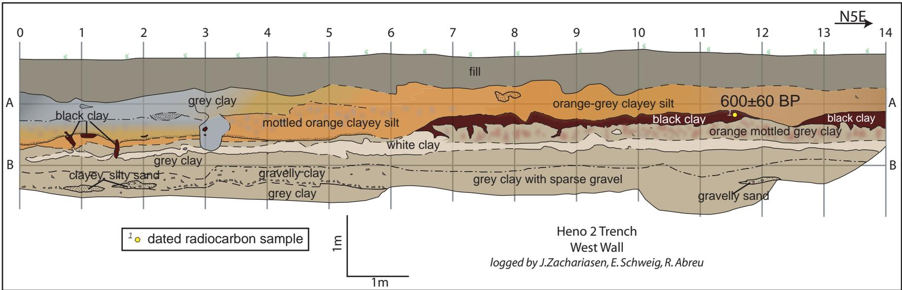
Figure 10. Log of west wall of trench H2. Fluvial sediments have undergone soft-sediment deformation, but there is no indication of faulting in the trench. Radiocarbon age is conventional age.
