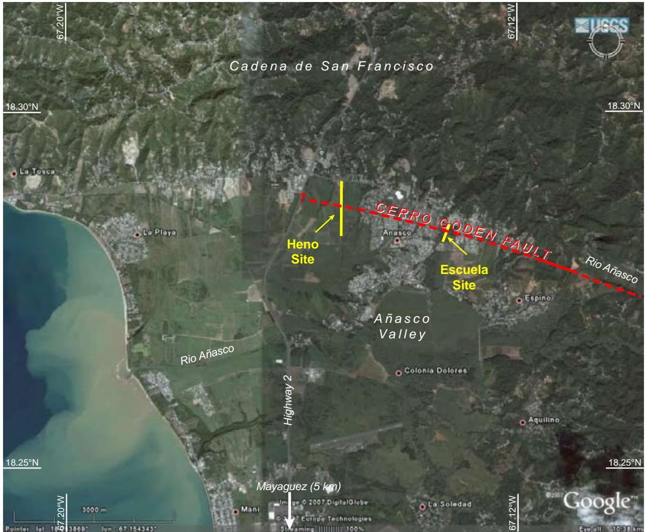
Figure 4. Añasco Valley. Red line depicts the Cerro Goden fault, solid where it occurs in bedrock exposures, and dashed where inferred in Quaternary alluvium. Note that the range front escarpment is several hundred meters north of the mapped fault, implying significant scarp erosion and retreat. Also shown are Heno and Escuela study sites. Image from Google Earth.
