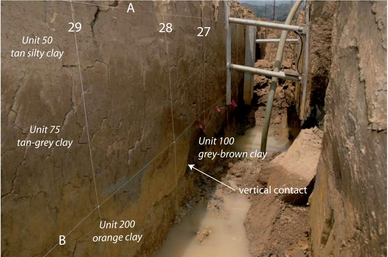
Figure 13. West wall of trench H4. View to northwest shows scarp in orange clay and dark grey to black organic-rich clay layers.
