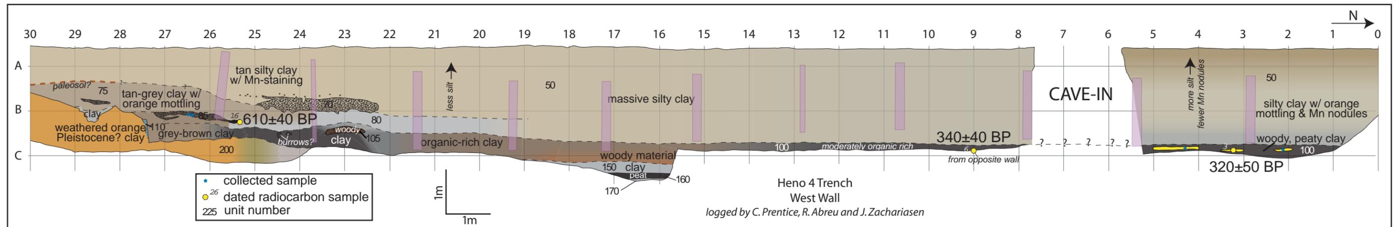
Figure 12. Log of west wall of trench H4. A subsurface scarp developed in highly weathered red clay appears in this trench. It is overlain by fluvial silt, sand and clay, as well as numerous lenses of black organic-rich, woody clay and peat. Radiocarbon ages shown are conventional ages.
