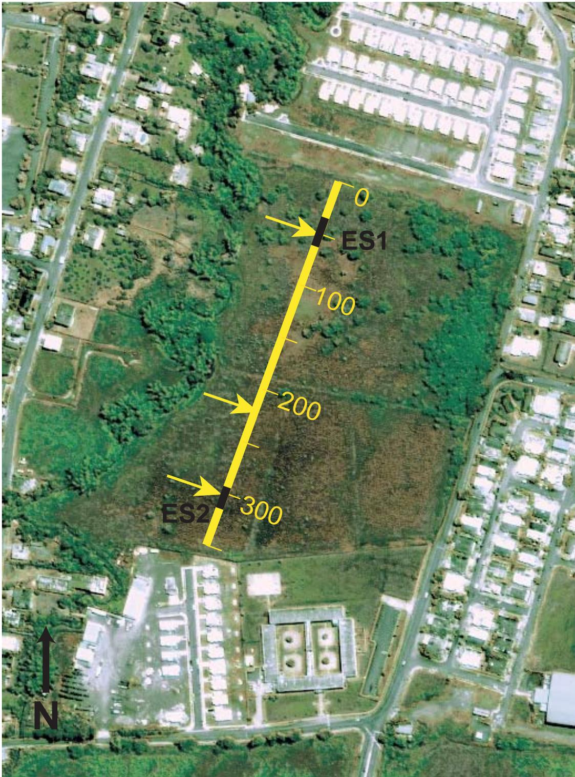
Figure 5. Satellite (IKONOS) image superimposed on 1936 air photo of the Escuela site, located northeast of Añasco. Scale marks seismic line. Trench locations indicated in black.
