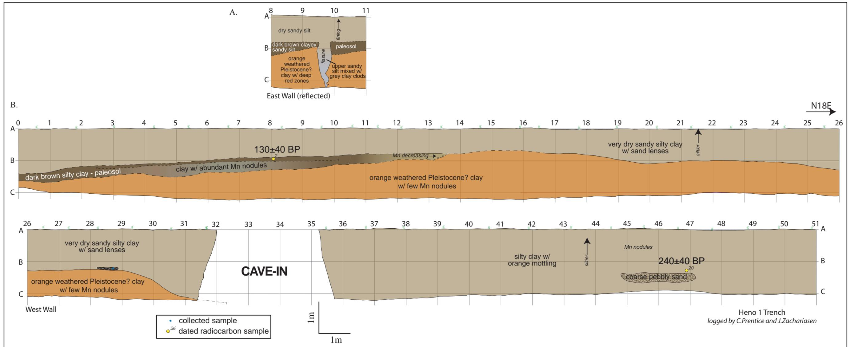
Figure 9. Log of west wall (B) and portion of east wall (A) of trench H1. Radiocarbon ages shown are conventional ages.
