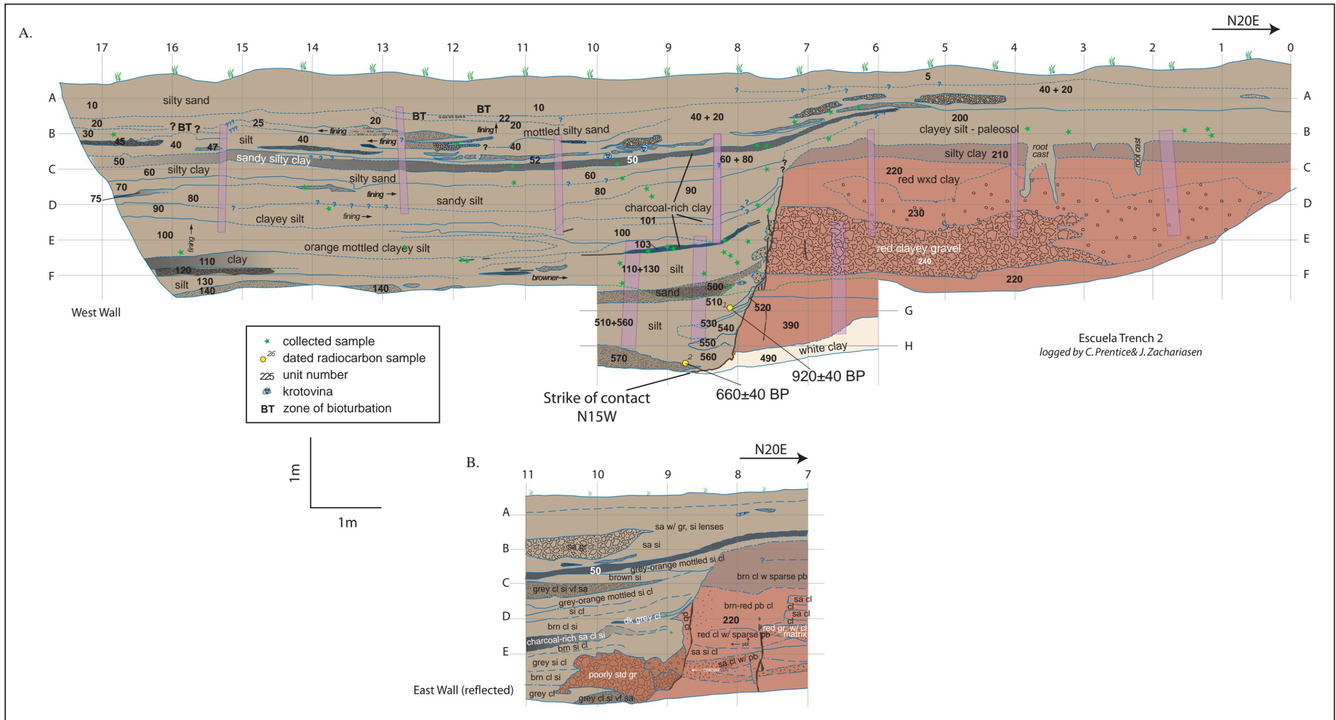
Figure 7. Log of trench ES2. a) West wall of trench. b) Central portion of east wall of trench, exposing subvertical contact between Holocene fluvial deposits and Pleistocene clay and weathered gravel. Dated samples show conventional radiocarbon ages.
