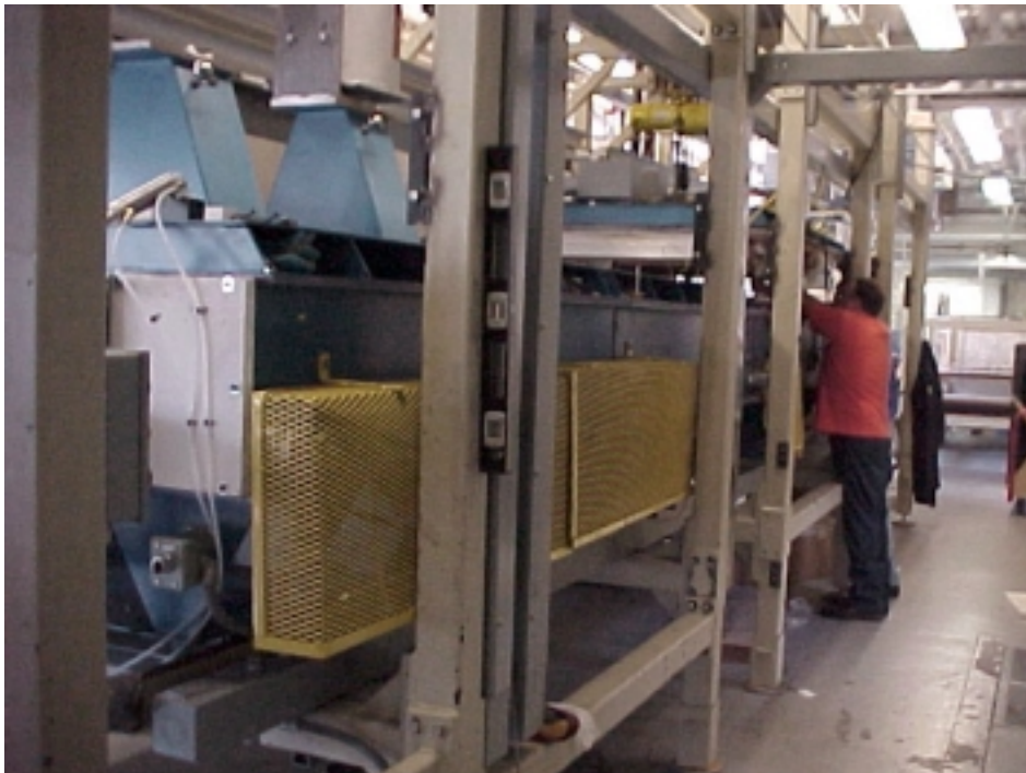
Figure 1.9 Large-area vapor-CdCl 2 treatment system
