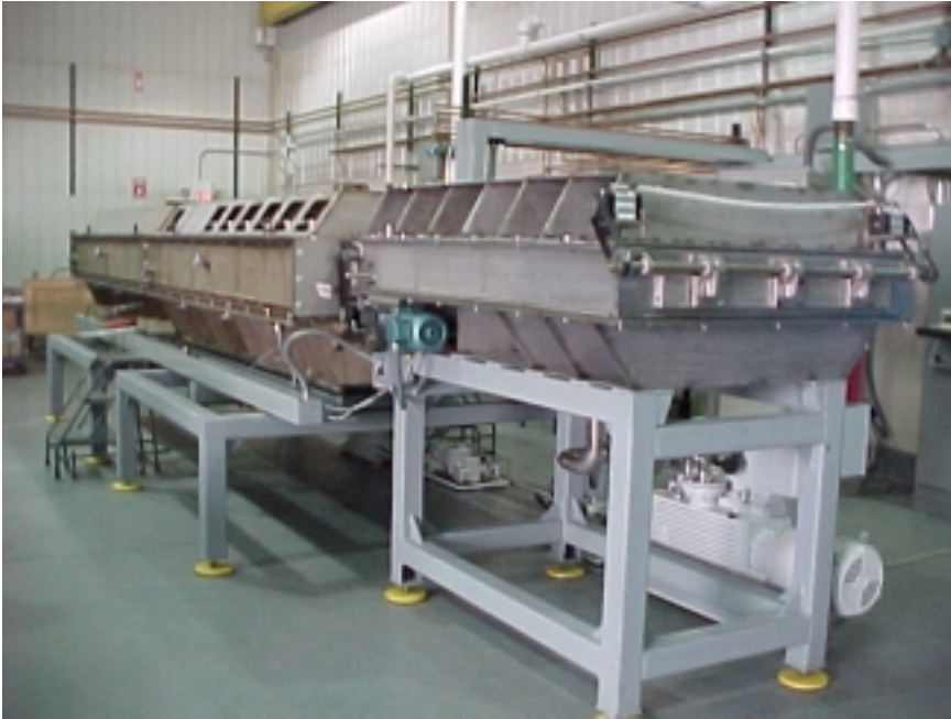
Figure 2.2 Large-area sputter deposition system for research.
