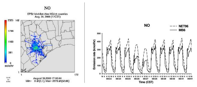
**Figure 4.** Spatial distributions of MOBILE6 NO emissions (left) and comparison of temporal emissions rates with NET96 (right).
