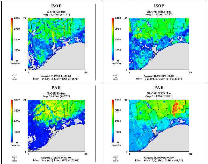
**Figure 5.** Comparison of ISOP (top) and PAR (bottom) emissions using GLOBEIS3 (left) and BEIS3 in SMOKE (right).
