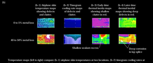
those same locations, (b-3) early-time thermal inertias (0.1 to 0.5 seconds) after flash heating at the locations, and (b-4) late-time thermal inertias (1 to 3 seconds after heating) for (top row) noncorroded or barely corroded (0 to 5% metal loss) aircraft skins and (bottom row) heavily corroded (40 to 50% metal loss).
